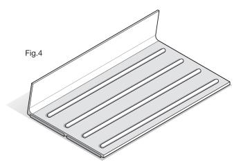
Place the stair edging so that the leading edge is overlapping the edge of the step and press down whilst sliding the profile into place. Press down firmly to ensure a full bond.
